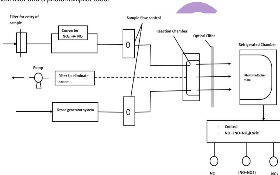
Figure 2: Chemiluminescence Analyzer
